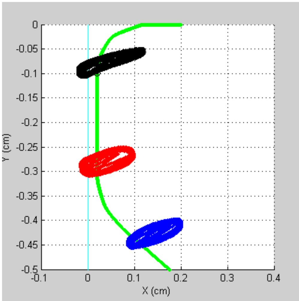
Figure 2. For the conditions of Figure 1, these are the trajectories of the three masses of the vocal fold. The outline of the vocal fold is given, as well as the prephonatory distance away from midline.
