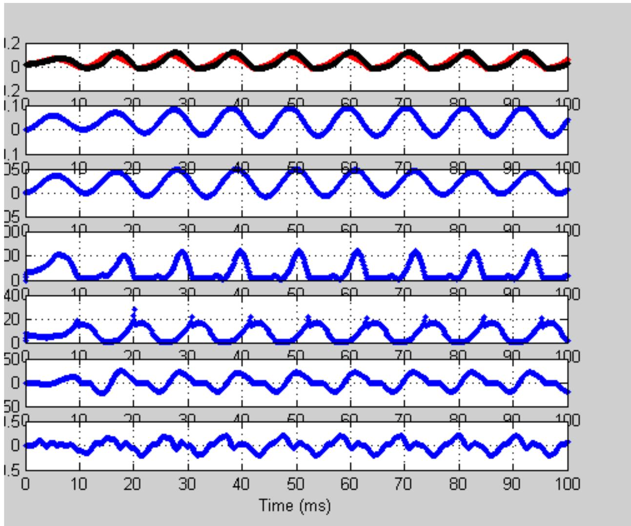
Figure 3. This figure, from top to bottom, is (1) the horizontal displacement of the two glottis-proper masses (like in the 2-mass models), (2) the horizontal displacement of the lowest (subglottal) mass, (3) the vertical displacement of the vocal folds, (4) the resultant laryngeal flow, (5) the transglottal pressure, (6) the glottal angle (positive is divergent, negative is convergent), and (7) the acoustic pressure at the lips (ala Ishizaka and Flanagan).
