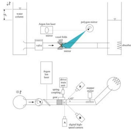
Fig. 1: Front- and top view of the experimental set-up
