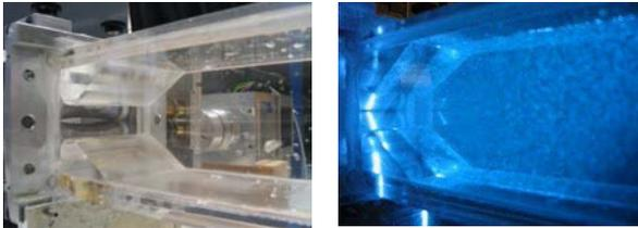
Fig. 6: Oblique photographic view upon the vocal folds unit through the unfilled channel (left) and under experimental conditions
