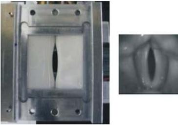
Fig. 3: Photographic view of the glottal model developed for this study (left) vs. laryngoscopic view of the human vocal folds at maximum opening (right, taken from <http://www.phoniatrie.uni-erlangen.de>)
