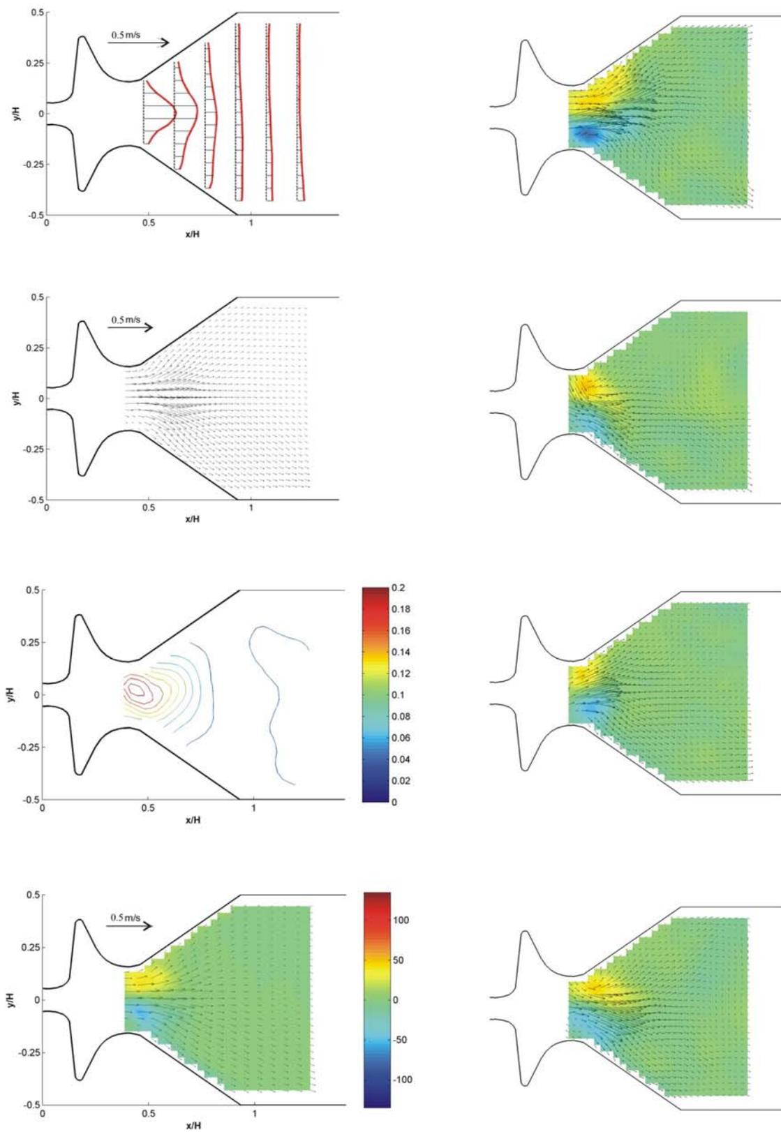
Fig. 8: Phase-averaged flow field (left column) and exemplar instantaneous pictures (right column) downstream of the glottis in the midplane at a given phase position in the vocal cycle: phase A.
