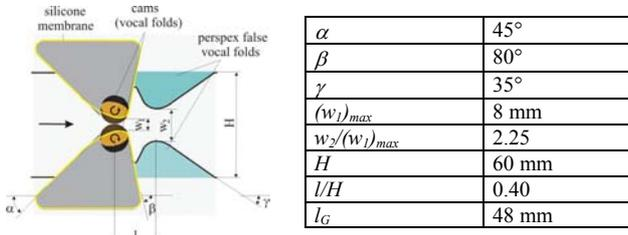
Fig. 5: Close-up view of a cut through the vocal folds unit and model dimensions
