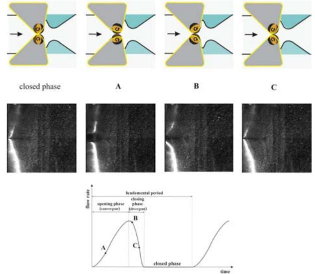
Fig. 7: Time dependence of the flow rate for one glottal cycle (bottom) and three selected characteristic phase points with respective cams angular position highlighted (middle and top).
